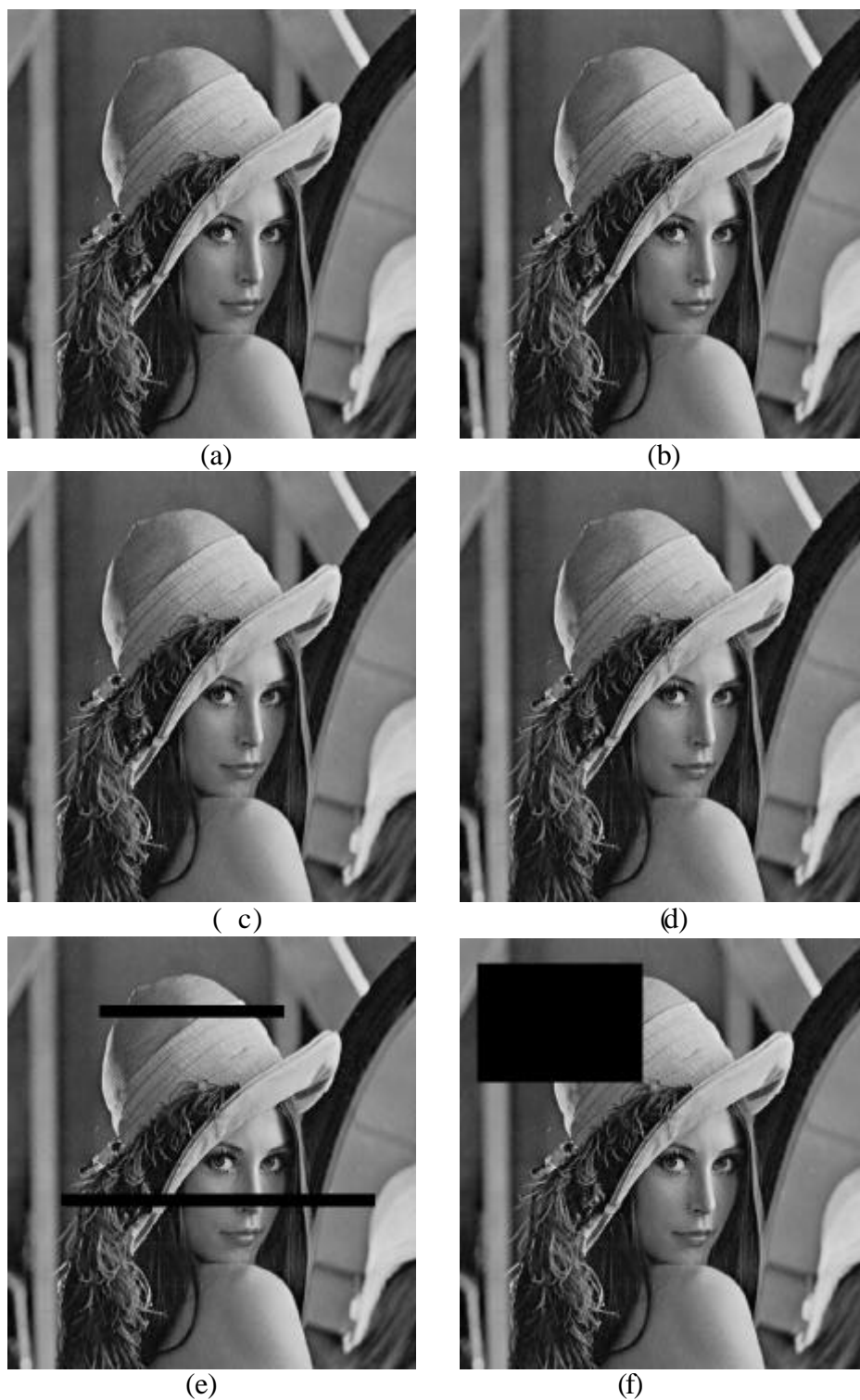
Figure 5. Test images for several attacks: (a) Original image; (b) Embedded image; (c) JPEG 90% quality; (d) JPEG 70% quality; (e) Painting; and (f) Cropping.
